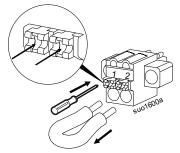
Push N/C relay contacts between the pins of the EPO connector until it is firmly connected. Use 0.5 to 1 mm<sup>2</sup> wire.
