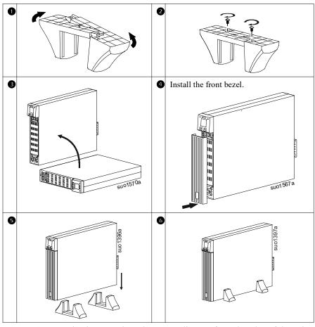
**NOTE**: Maintain approximately 70 mm distance from the edge of the unit, when installing the stabilizer brackets to the Easy UPS.
